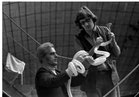
Figure 5. Frei Otto (left) with Eberhard Haug, Pneumatic experiment with inflated animal intestines, 1973 (photo IL Archive).
