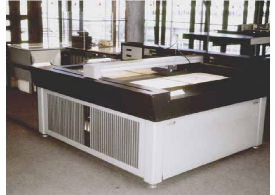
Figure 8. Zuse Graphomat 64 plotter on display at Expo '67, Montreal, 1967 (Horst Zuse).
